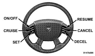
**NOTE:** The Electronic Speed Control System has been designed to shut down if multiple speed control switch buttons (i.e. SET and CANCEL) are operated simultaneously in order to ensure proper operation. The system can be reactivated by pushing the speed control switch ON/OFF button and re-establishing the desired vehicle SET speed.
